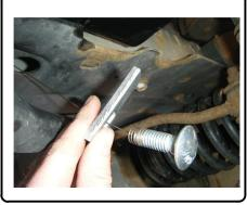
5. Slide hitch ,center section, inbetween slide plates, use 7/16" carriage bolts and nuts, to connect to side plates.
