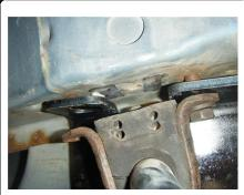
Locate back slot in passenger side plate and drill 1/2" dia. hole into frame.
