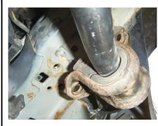
2. Slide drivers side plate into place, inbetween frame and bushing retaining bracket. Reinstall the 12mm bolts. Leave hardware loose until all bolts are installed.
