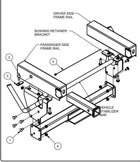
1. Remove front stabilizer bar bushing retaining bolts (save bolts for reinstallation)
